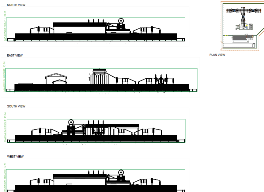
Figure 5-11: Sunnica East Site B Substation Elevation – 132kV solution (illustrative) (See Figure 3-11a of the Application [EN010106/APP/6.3])
